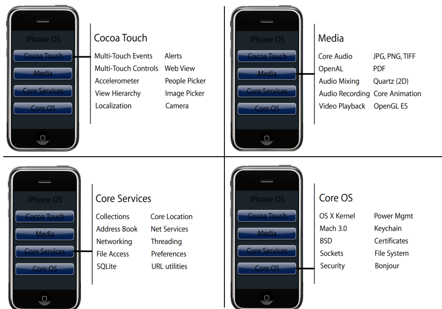
Figure 2.7: Detailed iOS Architecture (source: CS193P lectures, Stanford University)
